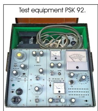
For regular maintenance and repairs of the VXW 100 (and many other VHF FM radios) a test set Tesla PSK 92 was used.
