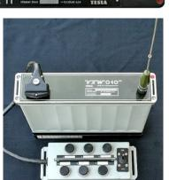
A spin-off from the VXW 100 was the VAW 010, a transmitter only, used for <u>remote control</u> of industrial and agricultural applications (above).
