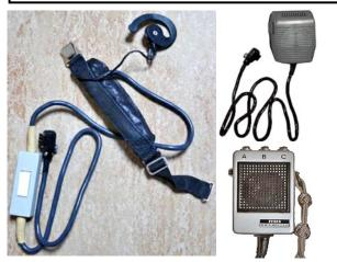
For (inconspicuous) hands free operation of the radio a throat microphone/ptt button and a short wire aerial could be used (left). QN 618 05 was the VXW 100 standard microphone (top right); the PX 25 microphone was primarily issued with the PR 11 (bottom right).
