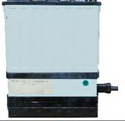
VYN 005 battery charger and rechargeable battery fitted at the bottom of a VXW 100 (left). It should be noted that the charger was only capable of charging, and could not be used to power a radio without a battery.
